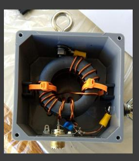
Workhorse UNUN 2 FT240-43 84-88% efficient 80-10M 85 W continuous, 212W CW. 340W SSB
