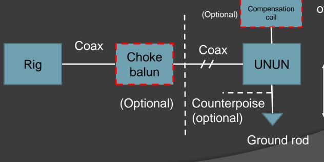
Inverted L shown (Recommended). Never run antenna wire next to a tower. Mount UNUN near top of tower instead.
