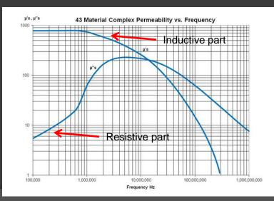
Permeability is actually complex - it has an inductive component (u') and a resistive (lossy) component (u'')
