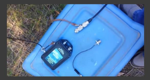
Disconnect UNUN from coax feed. Connect jumper between coax feed and antenna, leaving UNUN "float". The EFHW becomes a quarter wave antenna on 160 meters. Needs a good ground system to work properly.
