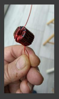
QRP UNUN >90% efficient 80-10M 5W continuous, 10W CW, 20W SSB
