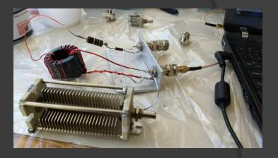
Test setup with 2 FT140-43 Small "QRP Plus" UNUN 80-10M 80-85% efficient 30W continuous 75W CW 120W SSB
