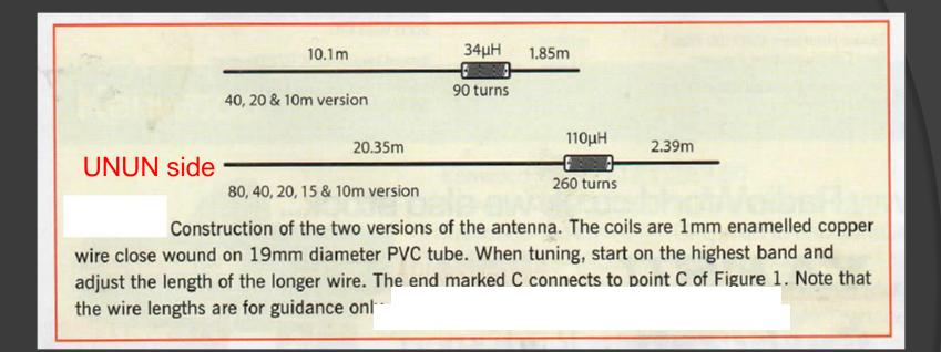
34uH coil: 90T, 110uH coil: 260 turns, 1mm (AWG #18) wire on 19m PVC tube. Adjust the long wire first for the high end bands. Then adjust the short wire for the lowest band.
