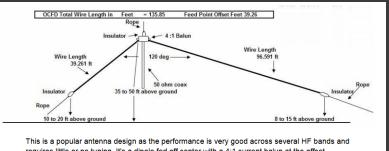
Inis a popular antenna design as the performance is very good across several HP bands and requires little or no tuning. It's a dipole fed off center with a 4:1 current balun at the offset feedpoint. The antenna shown covers 80, 40, 20 and 10 meters with 15 meters and WARC bands only available with an antenna tuner
