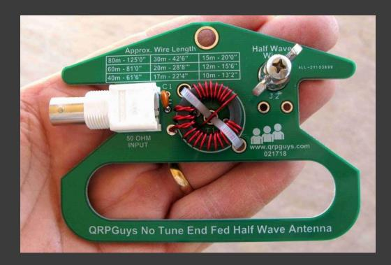
Low cost (\$15.00) Clever design for portable use. Rated <2:1 SWR, 10 watts
